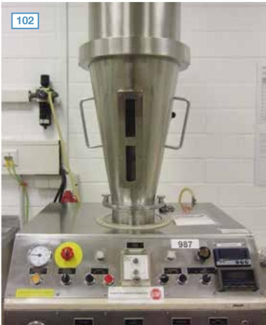
rotator-spraying-granulator, make: GLATT, type: UNI /
